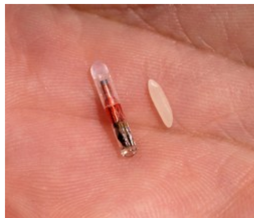
Figure 2. The VeriChip. A VeriChip is roughly the size of a grain of rice. Source: http://www.verichipcorp.com/
